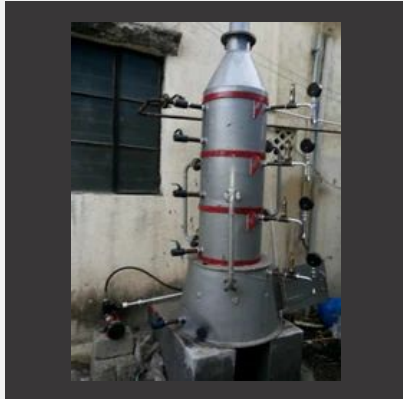
Automatic Steam Boiler
